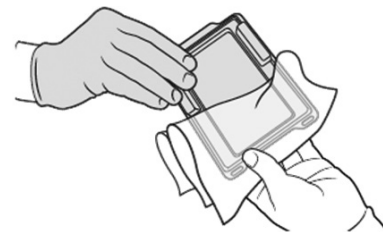
Figure 7: Sterile operator (gray gloves) removes the sterile Hold Dish presented by the nonsterile operator (white gloves)
